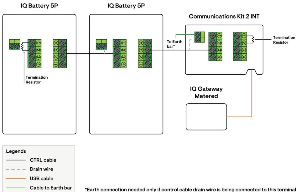
Sequence 2: IQ Battery 5P - Communications Kit 2 INT - IQ Battery 5P
